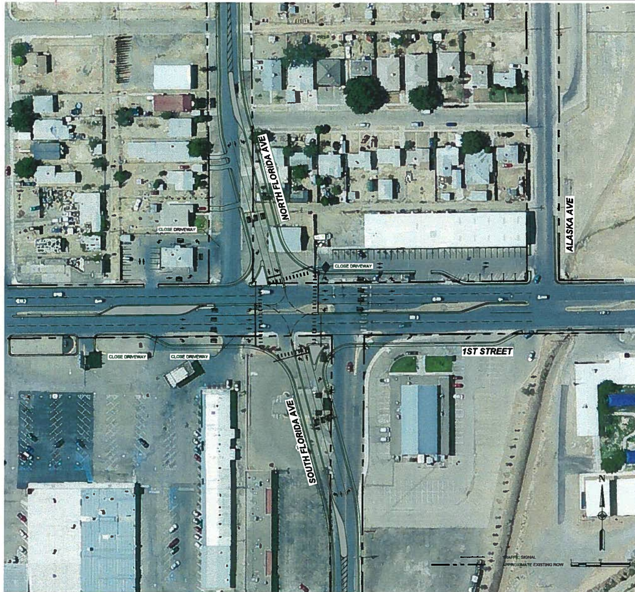
1 ALTERNATIVE II/III - SKEWED SIGNALIZED INTERSECTION
